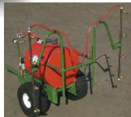
Trellis boom with 4 nozzle pipes on Nifty Pul Tank
