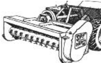
C - FL940 crop chop knife for heavy mowing and brush shredding
