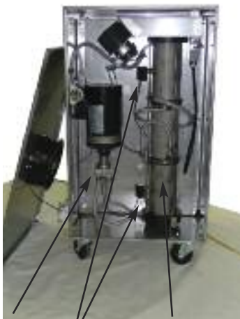
Pump Process tube UV sensors
