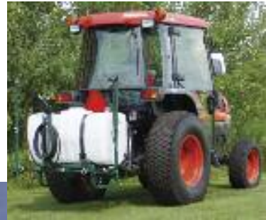
MSS P50 - 3 pt hitch sprayer, Cat #1 with R12M 12' boom
