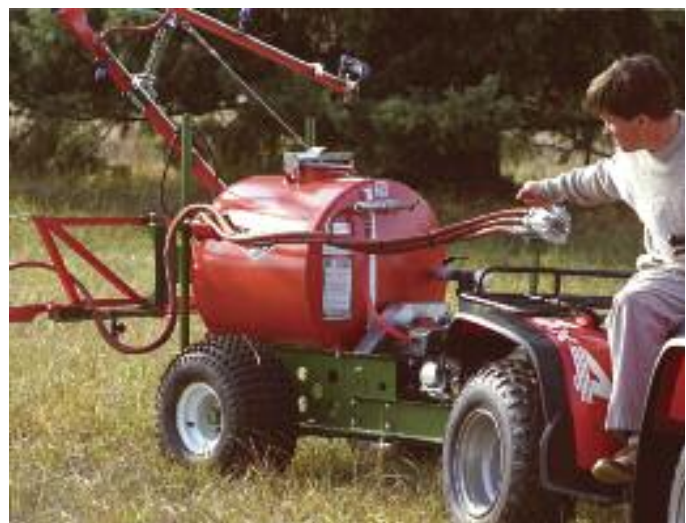
50 gallon Nifty trailer with flotation tires and Rears Nifty Boom
