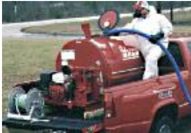
John Bean 300 gallon tank, 20 GPM pump
