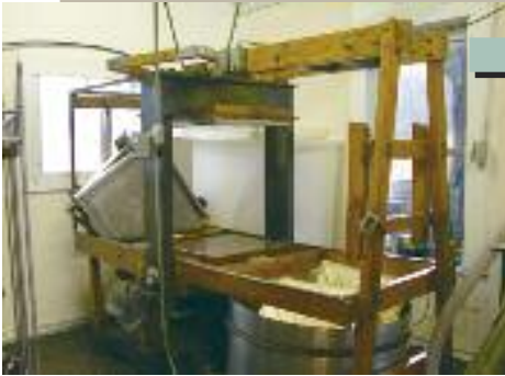
Wooden press - Palmer Design, manufactured by Orchard Equipment & Supply Co.
