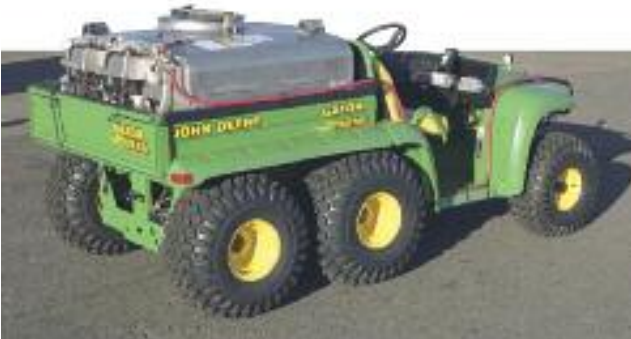
Rears 100 gallon 304SS low profile skid Honda engine Diaphragm pump
