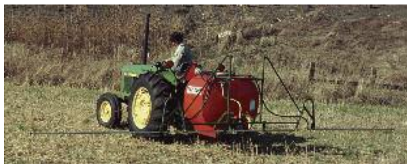
100 gallon Pak Tank with 3 section boom
