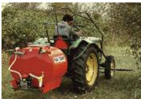
100 gallon Pak Tank with orchard weed boom
