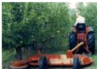
ZA 300 Rotary w/ Cutting Width 9'10"
