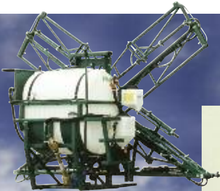
MSS P950E - with 45' hydraulic boom
